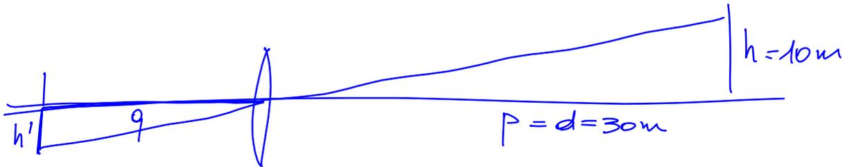
$$\frac{h'}{h} = \frac{q}{p} \quad h' = h \frac{q}{p} = 10\text{m} \frac{0.3\text{m}}{30\text{m}} = 0.1\text{m}$$
