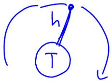
$$F_{\text{centrifuga}} = \frac{m v^2}{R_T + h} = F_{\text{gravità}} = G \frac{m M_T}{(R_T + h)^2}$$
