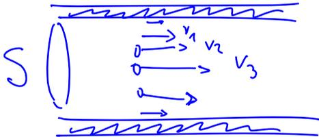
$$Q = \sum_i \sigma_i v_i \quad \text{portata}$$
